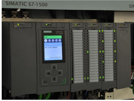
Figure 1: A hardware PLC of the S7-1500 series [23]
